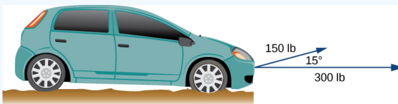
Figure 1.2.20: Two forces acting on a car in different directions.
