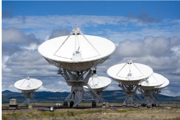
Figure 1.1.1: The Karl G. Jansky Very Large Array, located in Socorro, New Mexico, consists of a large number of radio telescopes that can collect radio waves and collate them as if they were gathering waves over a huge area with no gaps in coverage. (credit: modification of work by CGP Grey, Wikimedia Commons)
