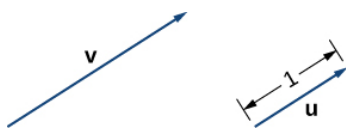
Figure 1.2.16: The vector \vec{v} and associated unit vector \vec{u} = \frac{1}{\|\vec{v}\|} \vec{v} . In this case, \|\vec{v}\| > 1 .
